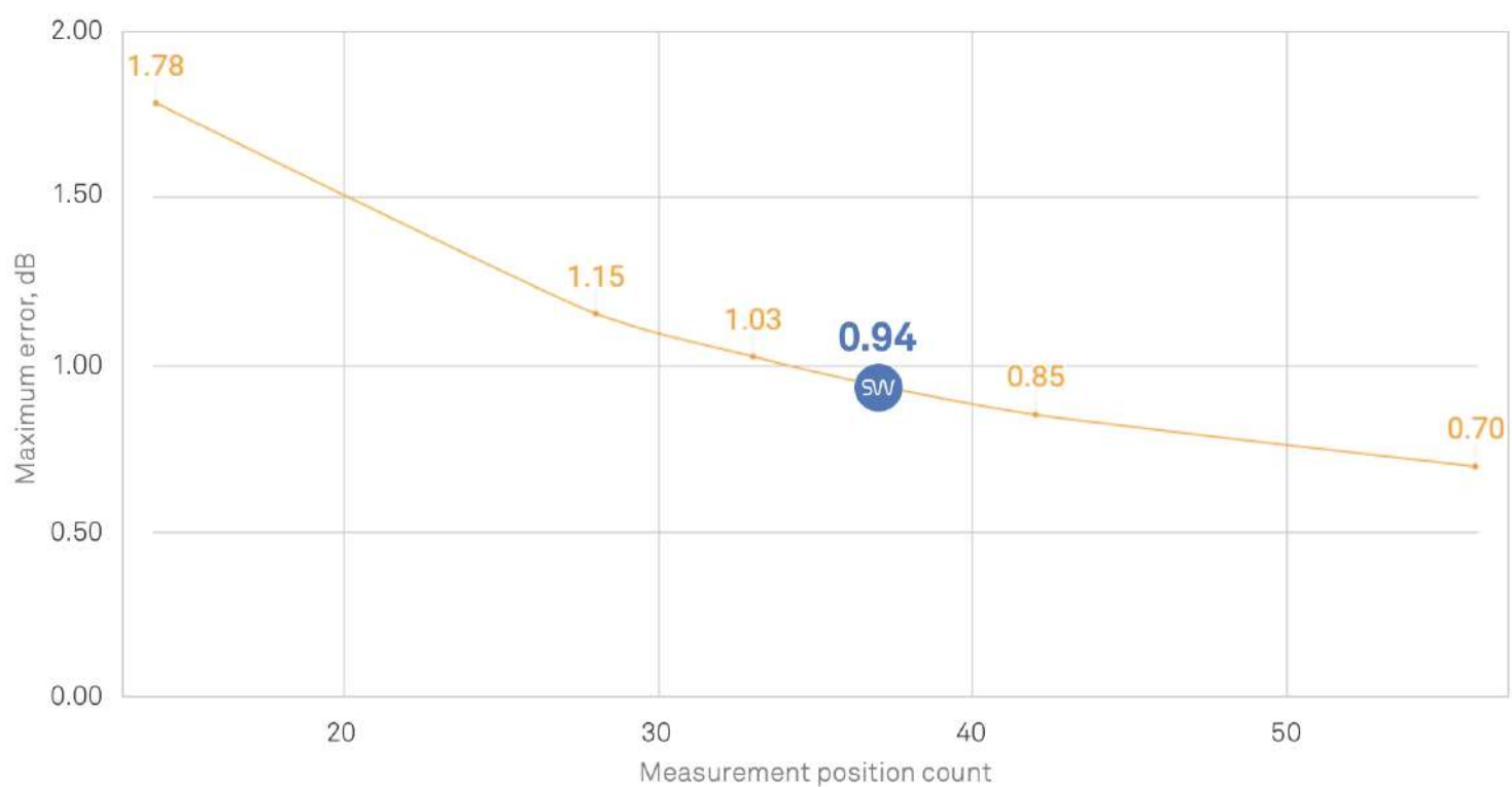
Figure 7: Sonarworks SR speaker measurement accuracy. A measurement of 37 points around the listening spot yields a maximum error of 0.94 dB
