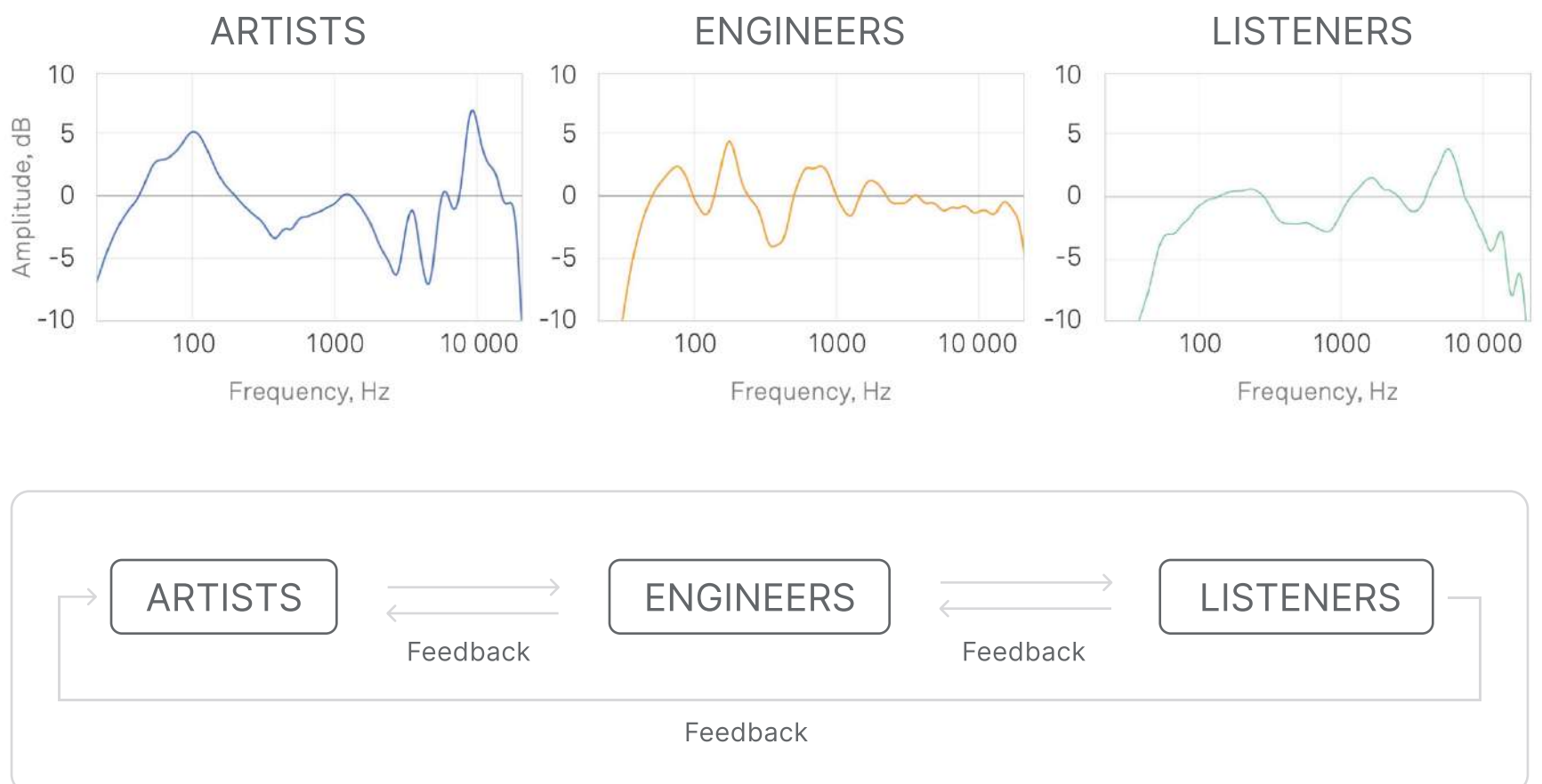
Figure 5: The cycle of compromise. Since nobody has access to a consistent sound standard, audio production is a continuous cycle of compromise
