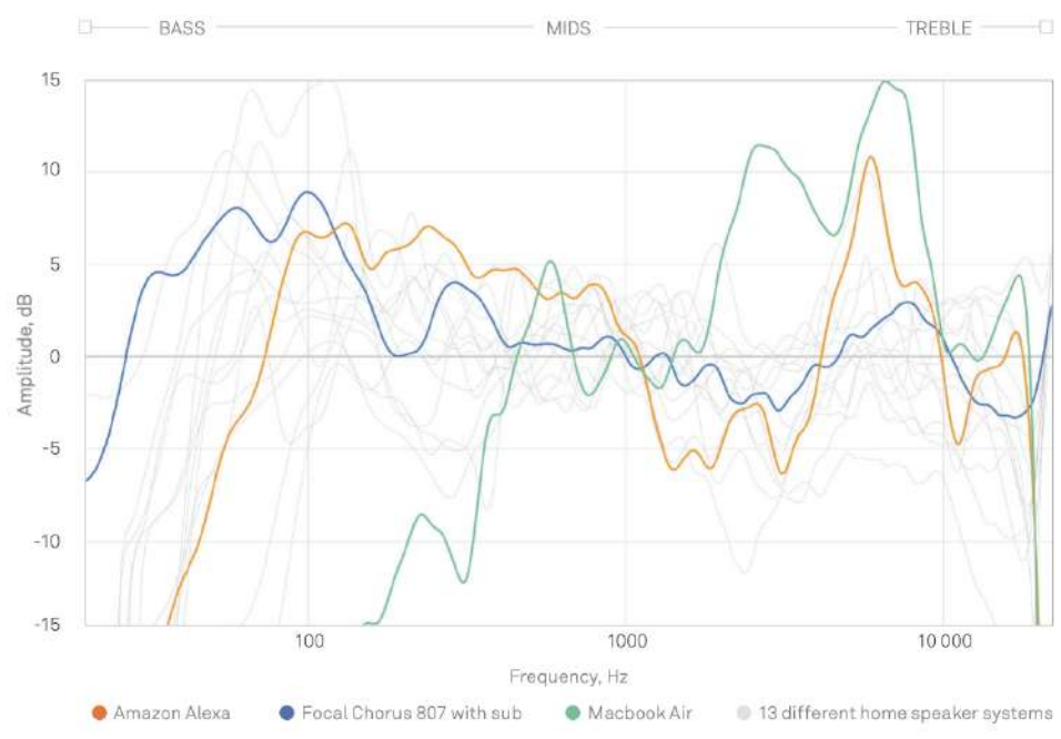
Figure 3: Frequency response variation of home speakers 16 home speaker pairs in various listening environments
